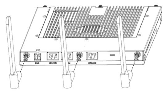
R1 defines the access point's radio 1 antenna connectors and R2 defines radio 2 antenna connectors.
