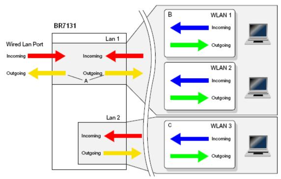
Adding a filter to LAN 1 for outbound traffic results in the inspection of packets at point A. Both packets out the physical port and wireless transmissions are checked. Adding a filter to WLAN 1 for inbound traffic results in the inspection of packets at point B. Even though WLAN 2 is on LAN 1, its packets are unaffected. Adding a filter to WLAN 3 for inbound traffic results in the inspection of packets at point C.
